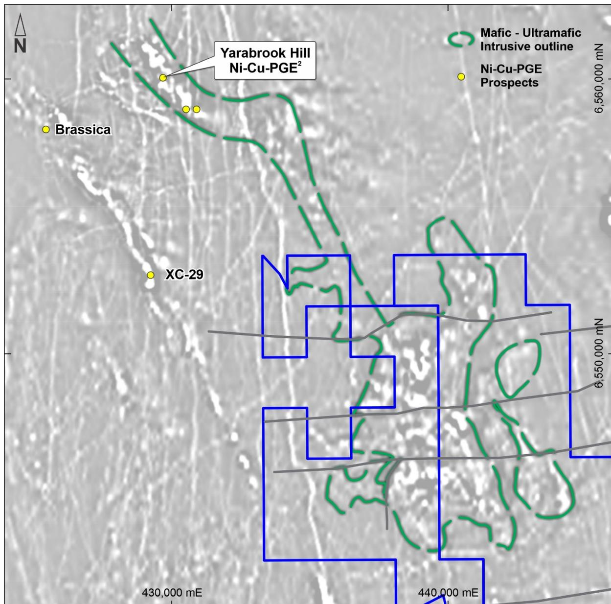
**Figure 3.** Sovereign Tenements and interpreted outline of mafic-ultramafic intrusion over airborne magnetics (1<sup>st</sup> vertical derivative) in relation to Caspian Resources Limited's (ASX: CPN) Yarabrook Hill Ni-Cu-PGE Prospect.
