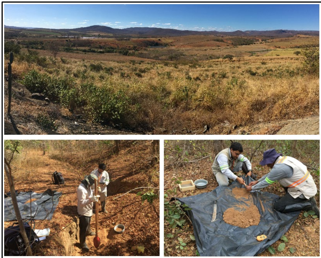
Figure 4: Stream sediment sampling, Salinas Lithium Project Brazil.
