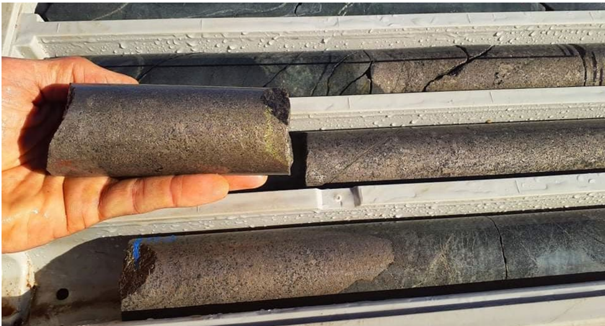
Figure 1. Photograph of massive sulphide intersected by NDD0003 from 111.6m to 113.5m downhole.
