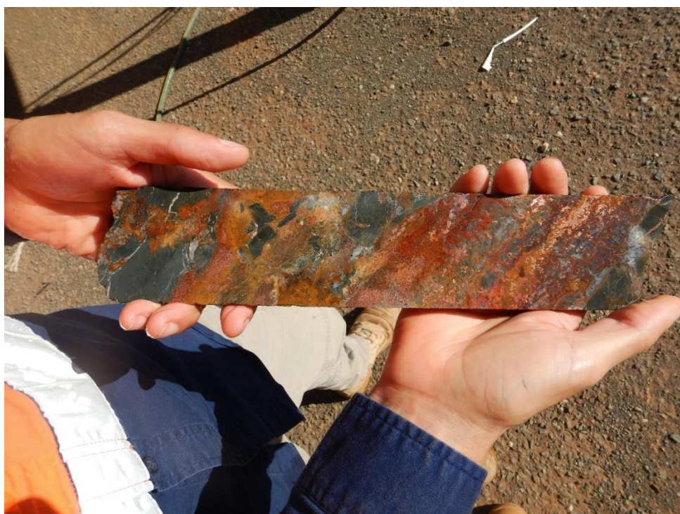
Figure 2: Hole 21CCDD003 122.36 - 122.66m chloritic altered brecciated basalt host with ~5% native copper with moderate to strongly oxidised limonite-goethite.
