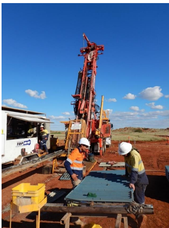
Figure 3: Truck mounted Sandvik DE880 drilling hole 21CCDD004 at Carlow Castle.
