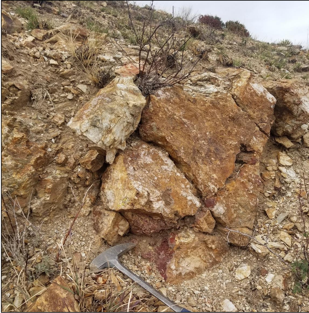
Figure 3 - Sample 41160 (1.62 g/t Au and 10.30 g/t Ag). Vuggy quartz vein with pods of massive hematite, jarosite and goethite on fractures at old prospect.
