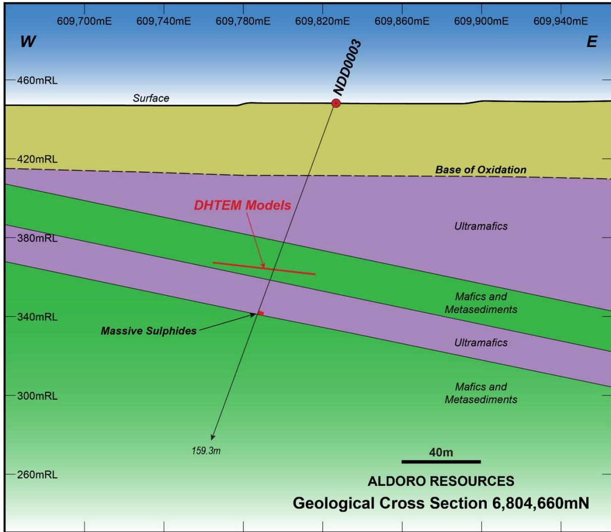
Figure 3. Cross-section of NDD0003 at 6804660m north (MGA50)
