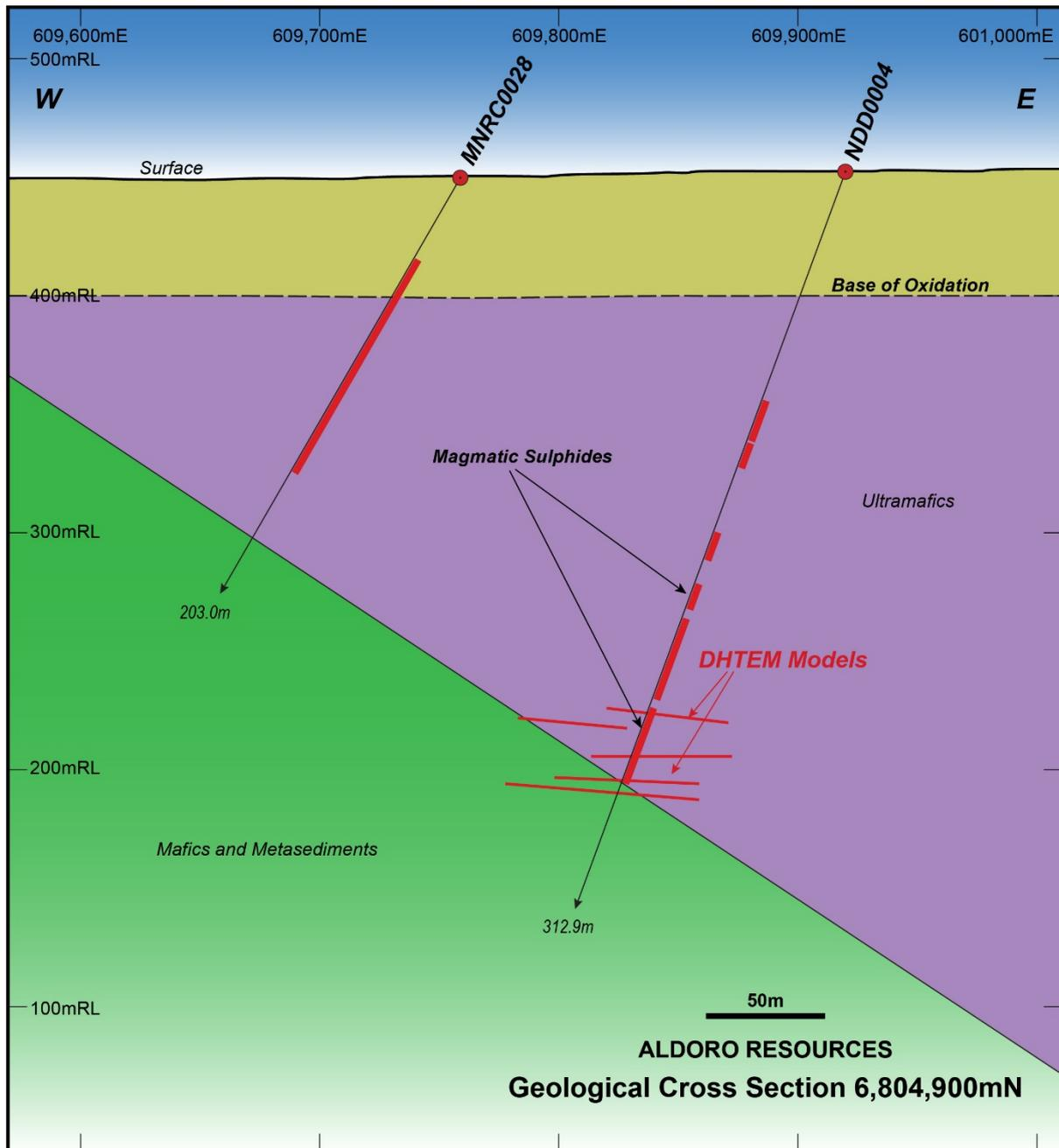
Figure 6. Cross-section of NDD0004 at 6804900m north (MGA50)
