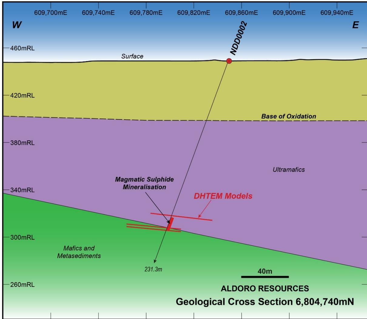
Figure 4. Cross-section of NDD0002 at 6804740m North (MGA50)
