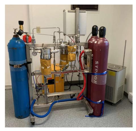
**Images:** State of the art CO<sub>2</sub> Supercritical Extraction System from Advanced Extraction Systems Inc. at Halucenex's onsite laboratory
