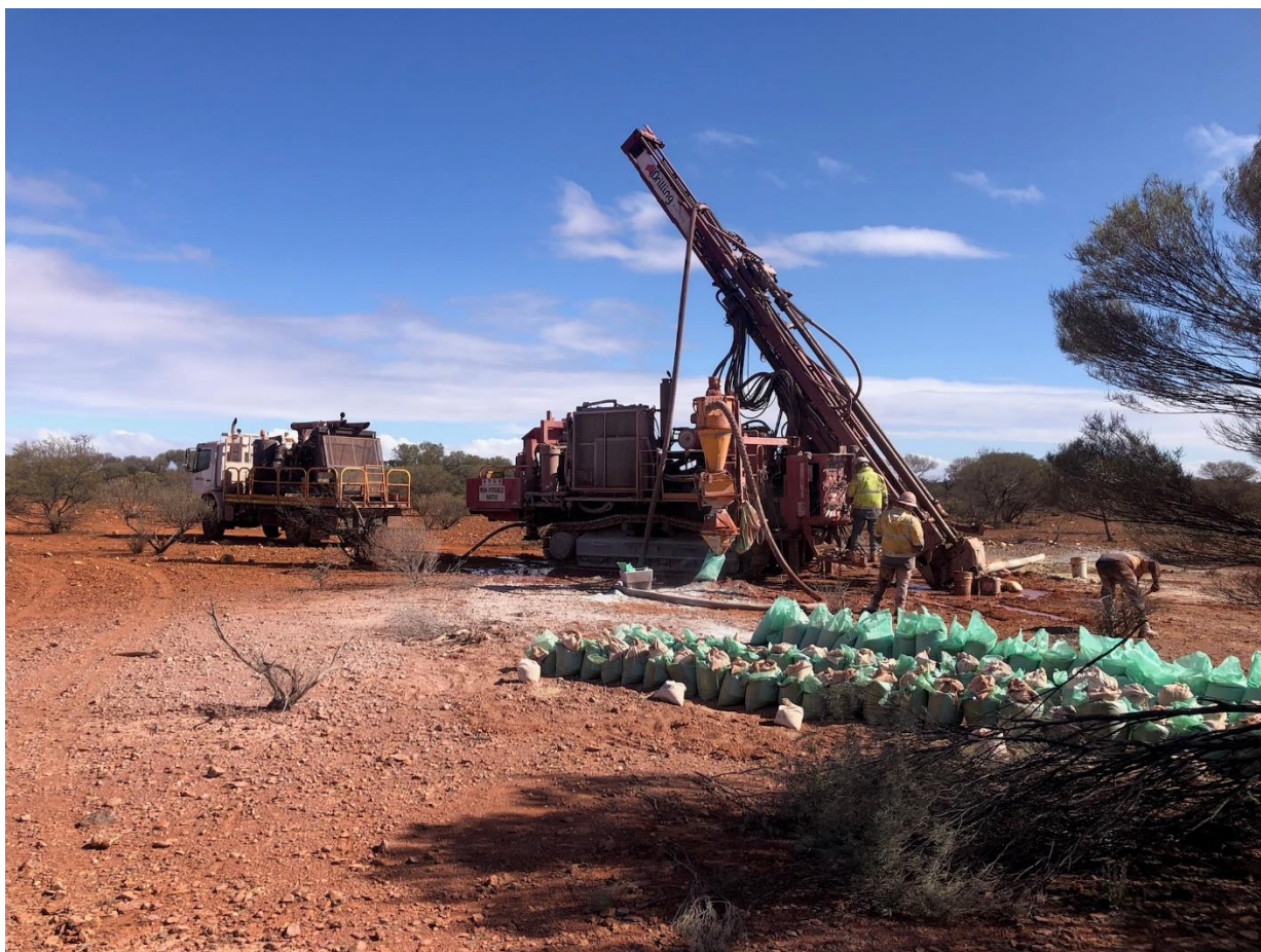
Figure 1: RC drill rig on site at Pharos
