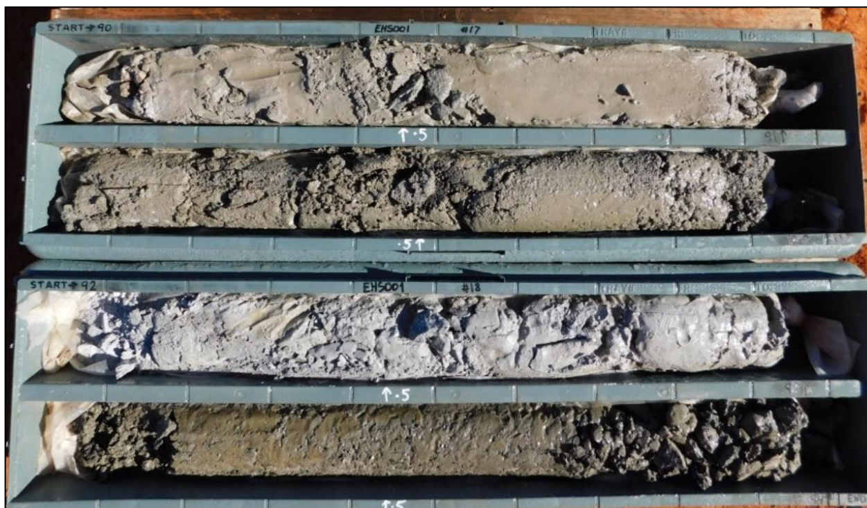
Figure 2 – Mineralisation Zone –Sonic Drilling Core – EHS001 (twin of EHRC050). Sphalerite, galena and pyrite mineralisation was logged in this soft primary zone.
