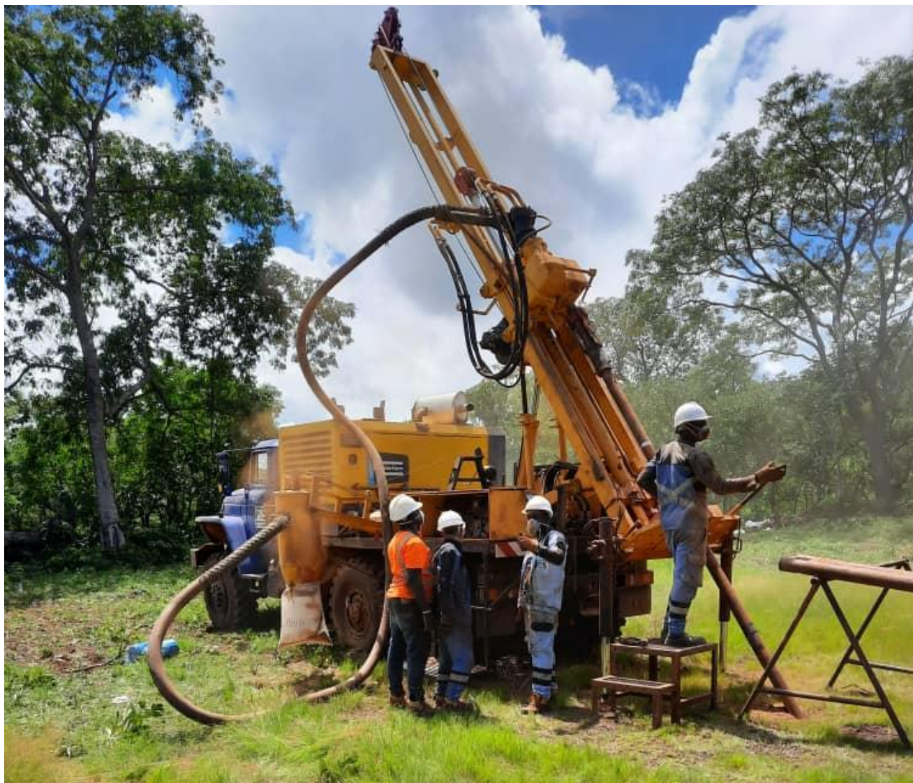
Figure 6 – Air Core drill rig on site at the NE Bankan Project, testing beneath gold anomalous zones identified by earlier power auger drilling.
