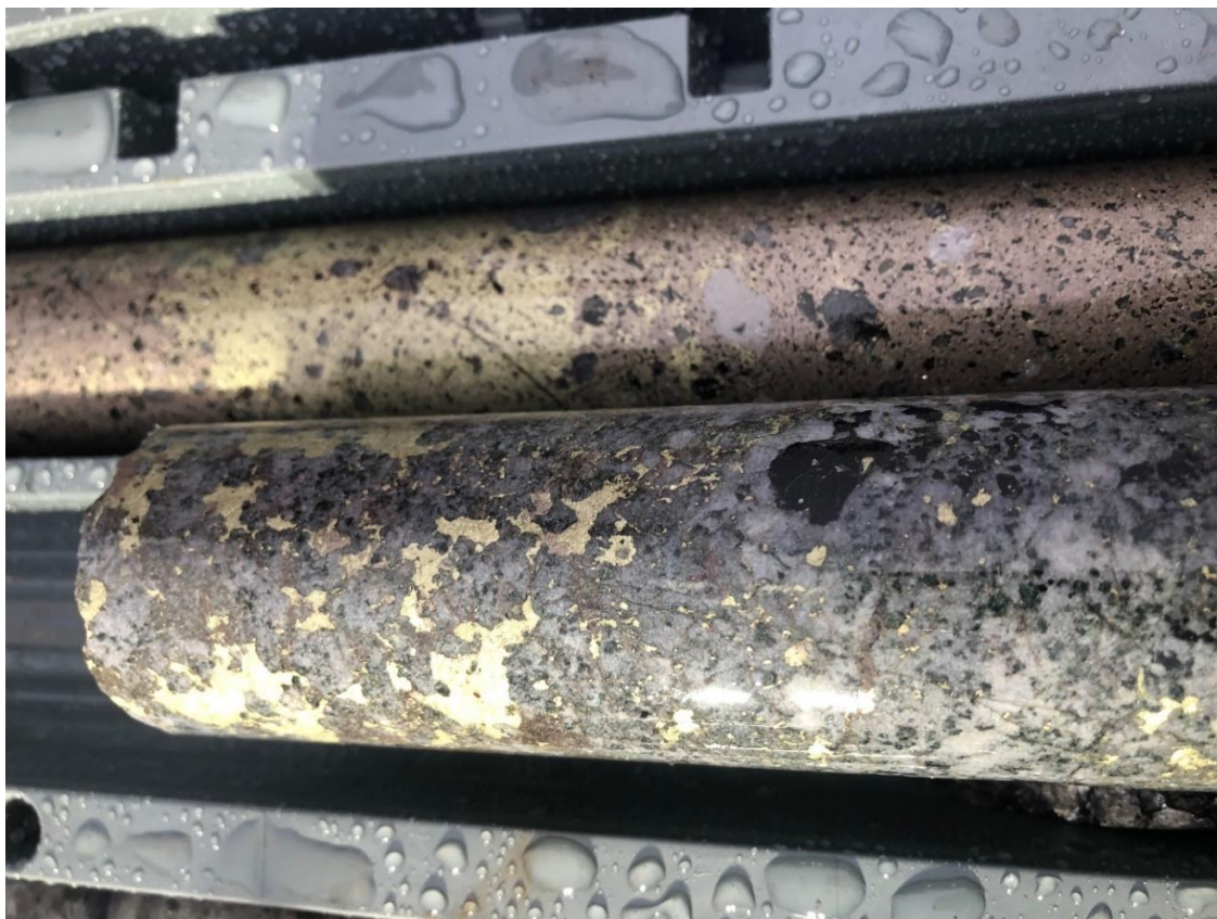
Figure 19 - 21PHDD002 Coarse-grained disseminated to blebby chalcopyrite and pyrrhotite in foreground and massive chalcopyrite and pyrrhotite with lesser arsenopyrite in the background.
