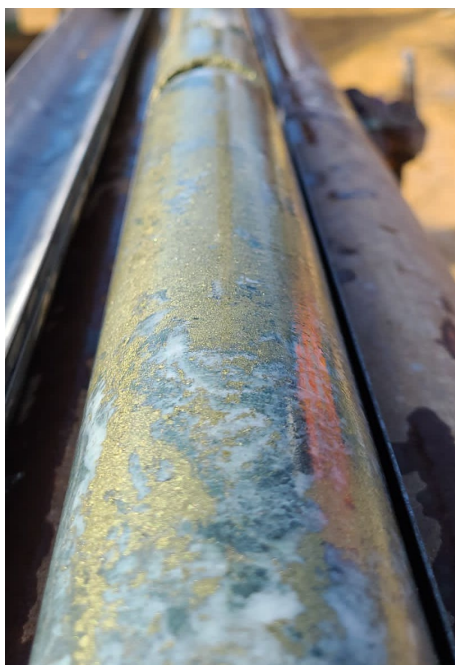
Figure 1: Drill Hole MCDD015 Showing Semi Massive Chalcopyrite Stringer
