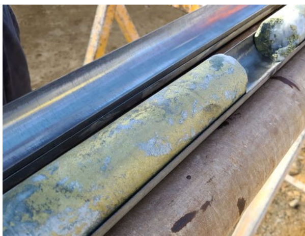
Figure 4: Drill hole MCDD015 showing semi massive chalcopyrite stringer veins.
