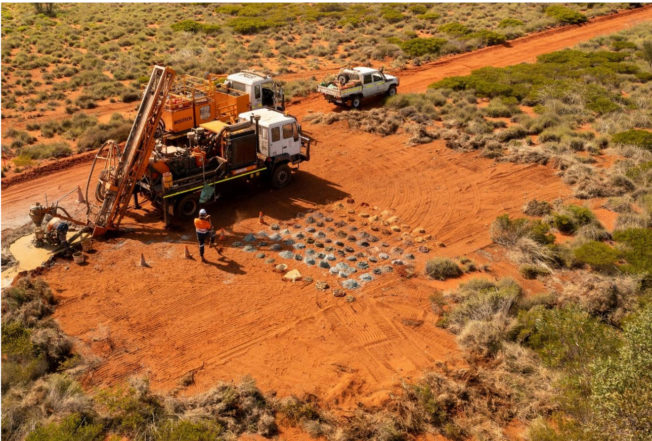
Figure 2: Air-Core Drilling at Roberts Hill
