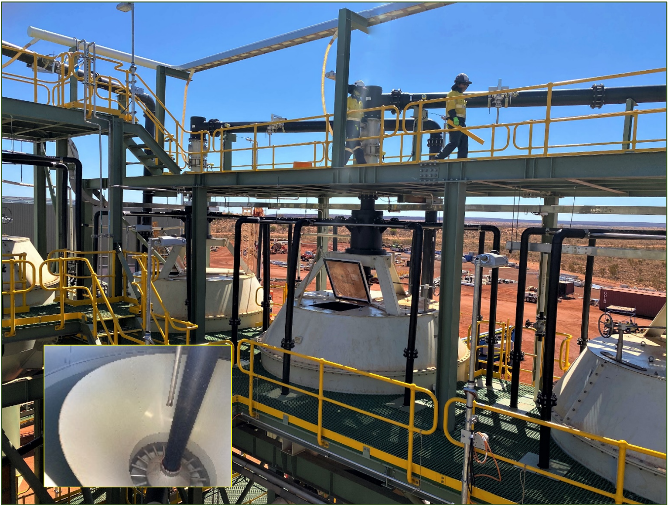
Flotation Circuit (inset shows inside of cell)
