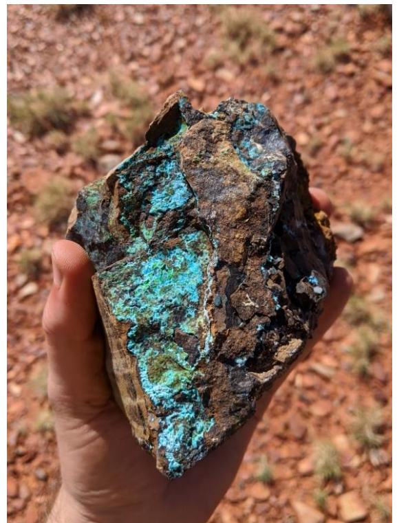
Photos: RC drilling rig (left) and copper-oxide mineralisation in gossan outcrop (right) at Hasties Prospect.
