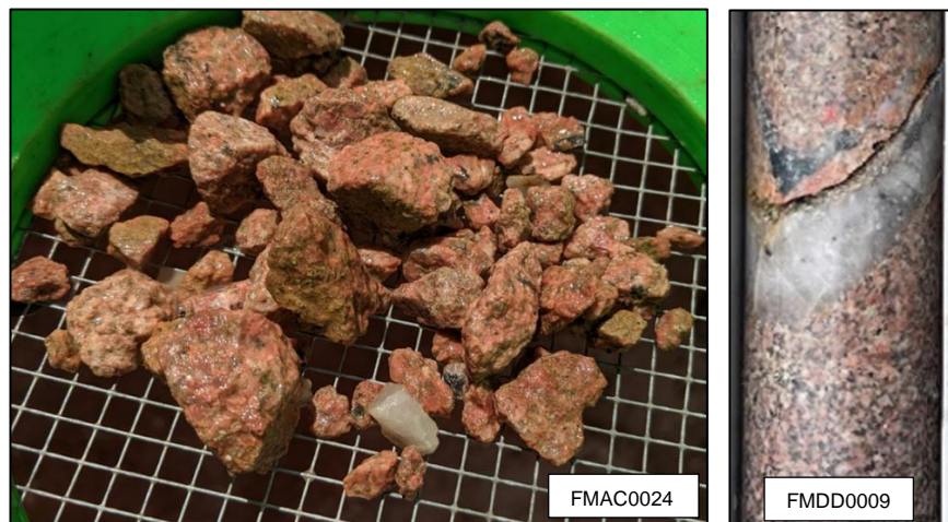
Figure 1: Early AC success in the drilling at Deep Well. The AC drilling has intersected quartz veining and associated hematite alteration with weathered sulphides (left). This is identical to intersections from the focussed diamond drilling (right), which is located several hundred metres to the south.
