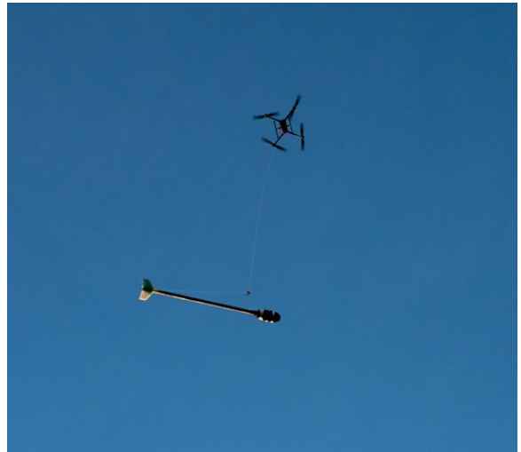
Newly available ultra-high resolution drone magnetic survey tools are providing very promising results in detecting subtle magnetic anomalies unseen by previous explorers.
