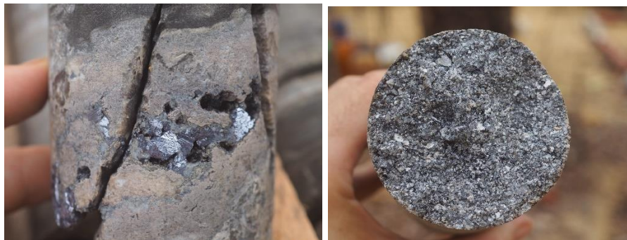
Coarse galena vein in NBDD018 and disseminated galena and sphalerite in NBDD006
