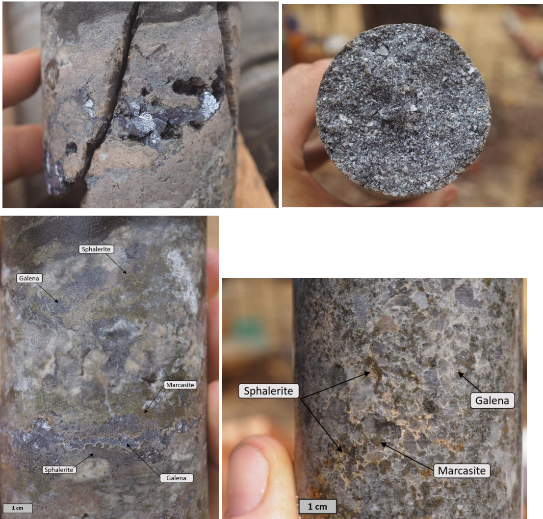
Figure 4 – Examples of mineralisation styles being encountered at Niamabimbo Coarse galena (lead sulphide) vein in NBDD018 within a dolostone at 34m (Top LHS). Disseminated galena and sphalerite (zinc sulphide) in sandstone (8% galena + sphalerite logged) in NBDD006 at 24m (Top RHS). Sphalerite (schalenblende style) and galena in NBDD016 at 23.5m (Bottom LHS). Sphalerite, galena and marcasite in sandstone within NBD014 at 18m (Bottom RHS)
