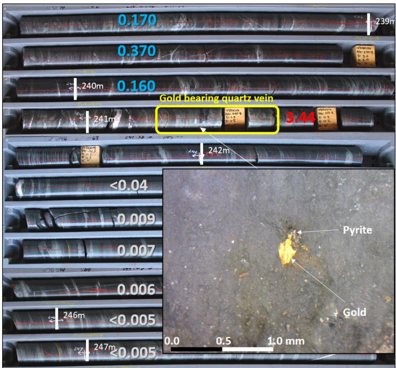
Figure 5; Photo of drillcore from hole VDD014 with annotated assay results showing grades up to 3.44g/t Au 241m. Note the distinct quartz veining and associated visible gold (yellow box).
