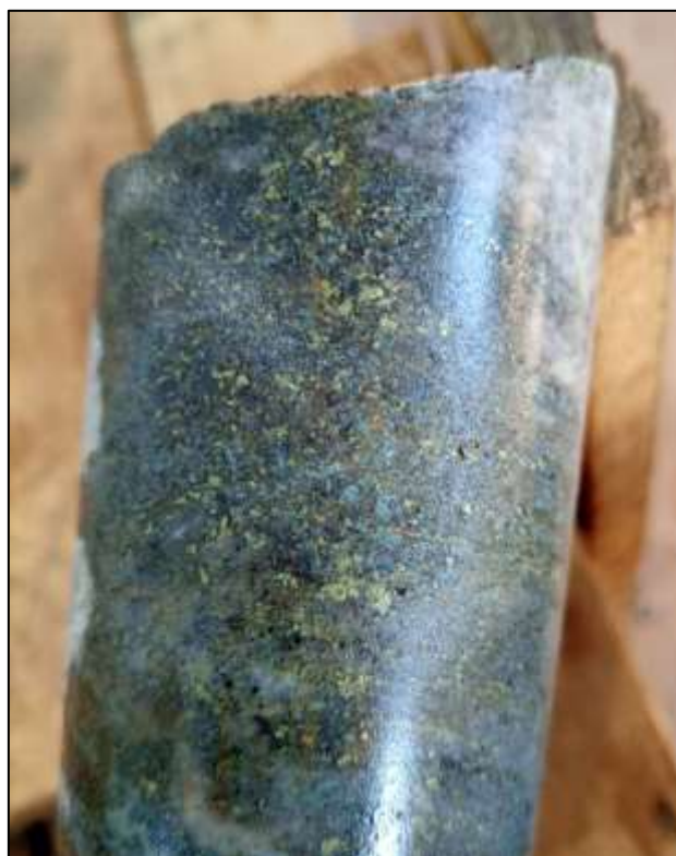
Figure 3 – Detail from CKDD003 exhibiting silicified metagranodiorite highly mineralised with chalcopyrite at 36m
