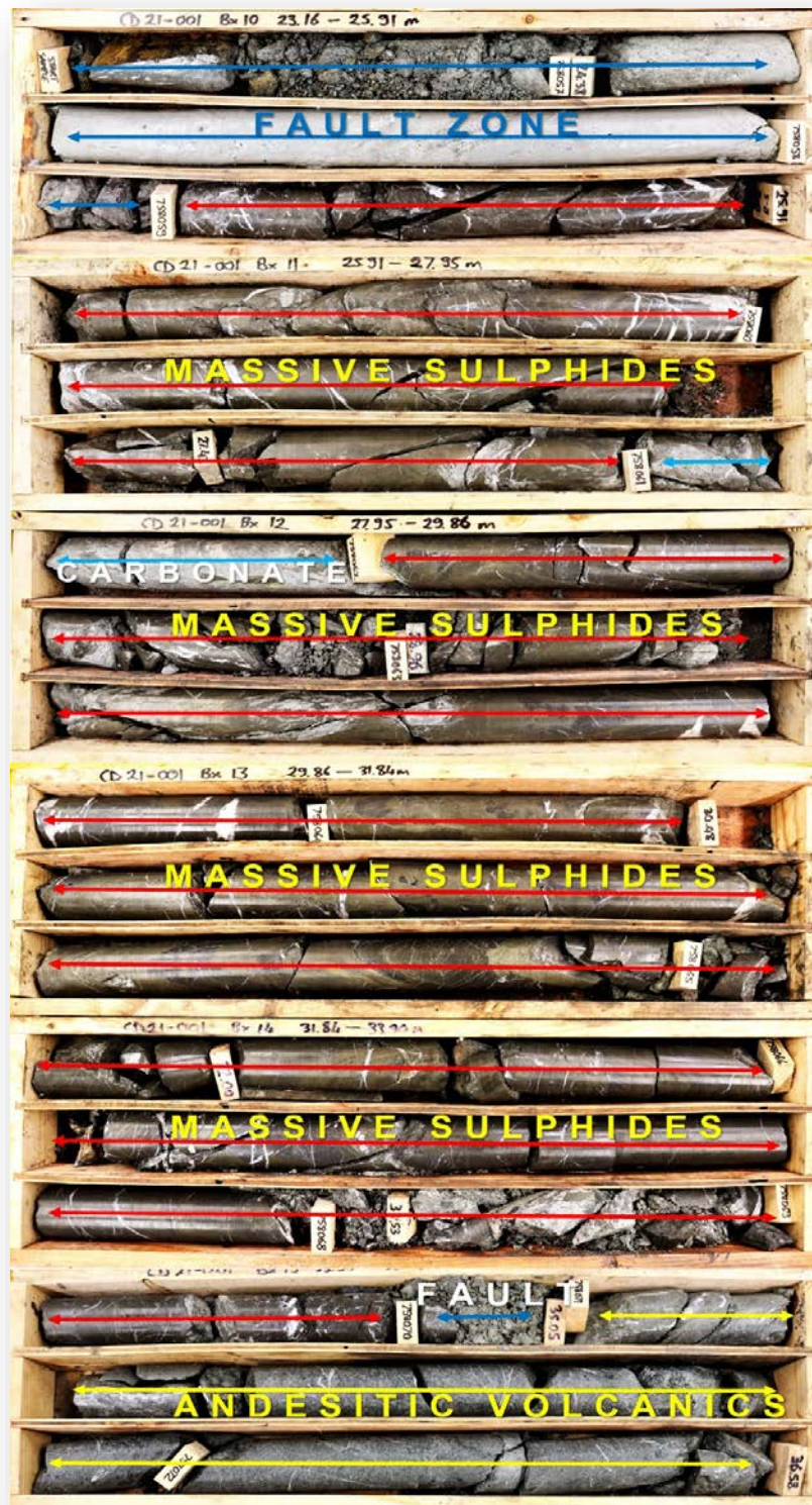
Figure 5 Core photos for hole CD21-001 between 23.16m and 36.58m showing the upper zone of massive sulphides intersected in this hole.
