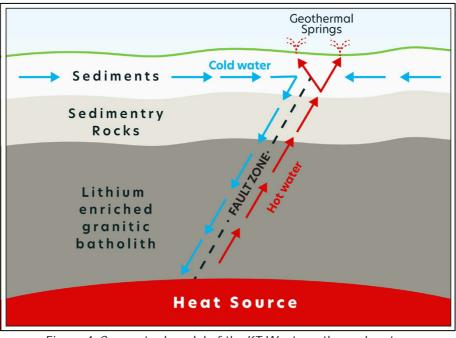
Figure 4: Conceptual model of the KT West geothermal system (modified from Ngansom and Duerrast, 2019)
