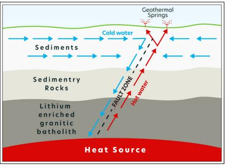
Figure 6: Conceptual model of the KT North geothermal system (modified from Ngansom and Duerrast, 2019)
