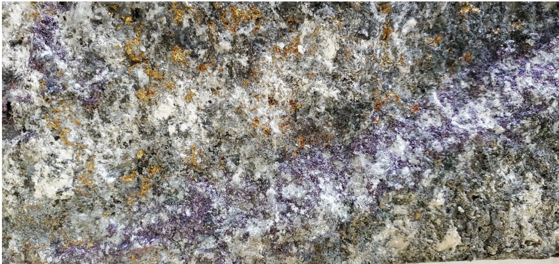
Figure 4 – Chalcopyrite and Bornite veinlet within the Leatherwood Intrusion (WT-21-22, 350.2m, photo is approximately 12 by 5cms)
