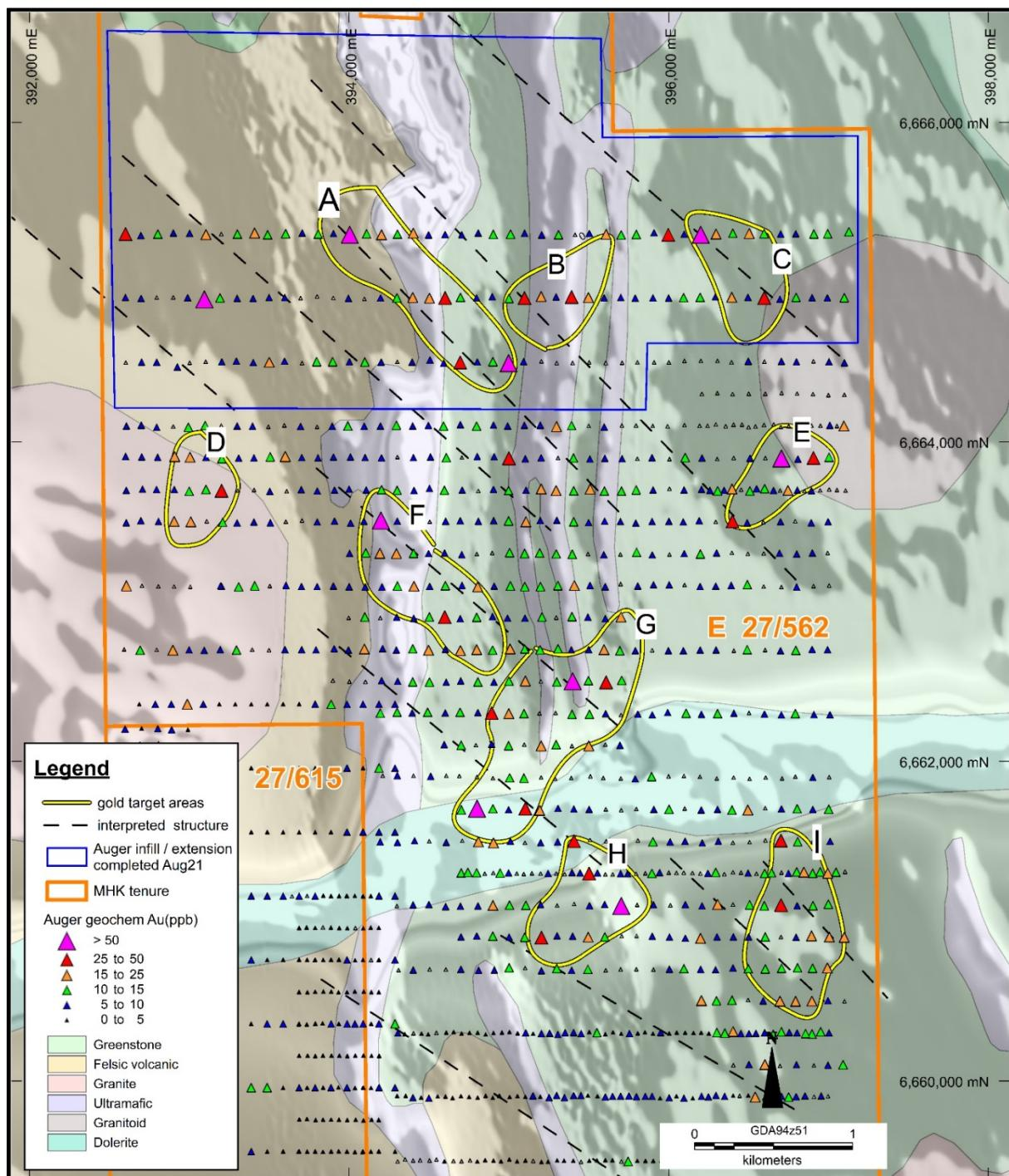
**Figure 3.** Emu Lake Project – geochemical and structural gold targets with auger drilling
