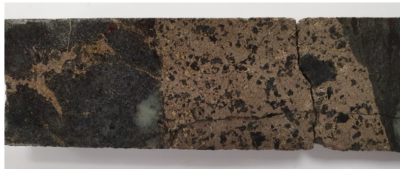
20WGDD005 340.4-340.5 ; Massive Sulphide ( remobilised)
