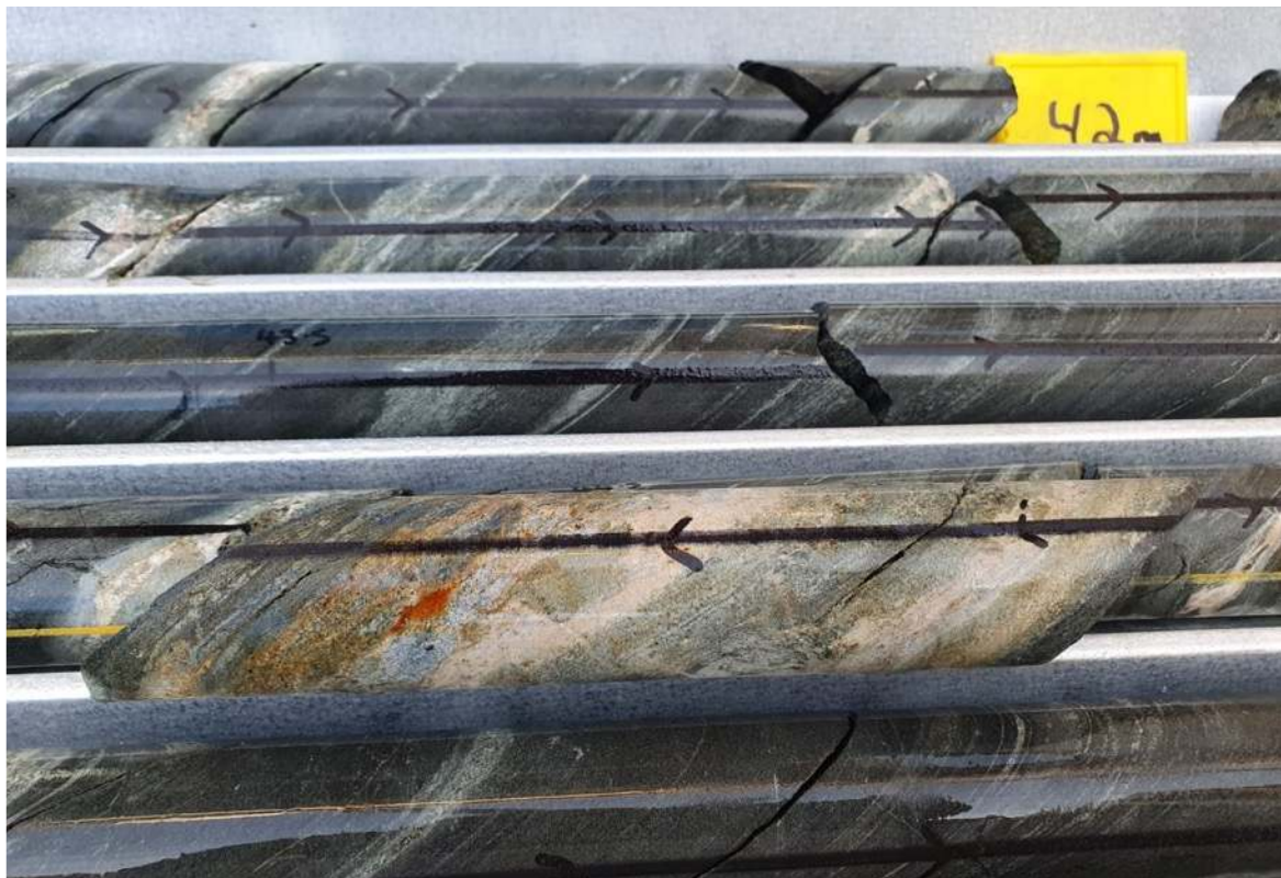
Figure 11: Amphibolite with oxidised sulphide (red) at 44m depth in SODD003.
