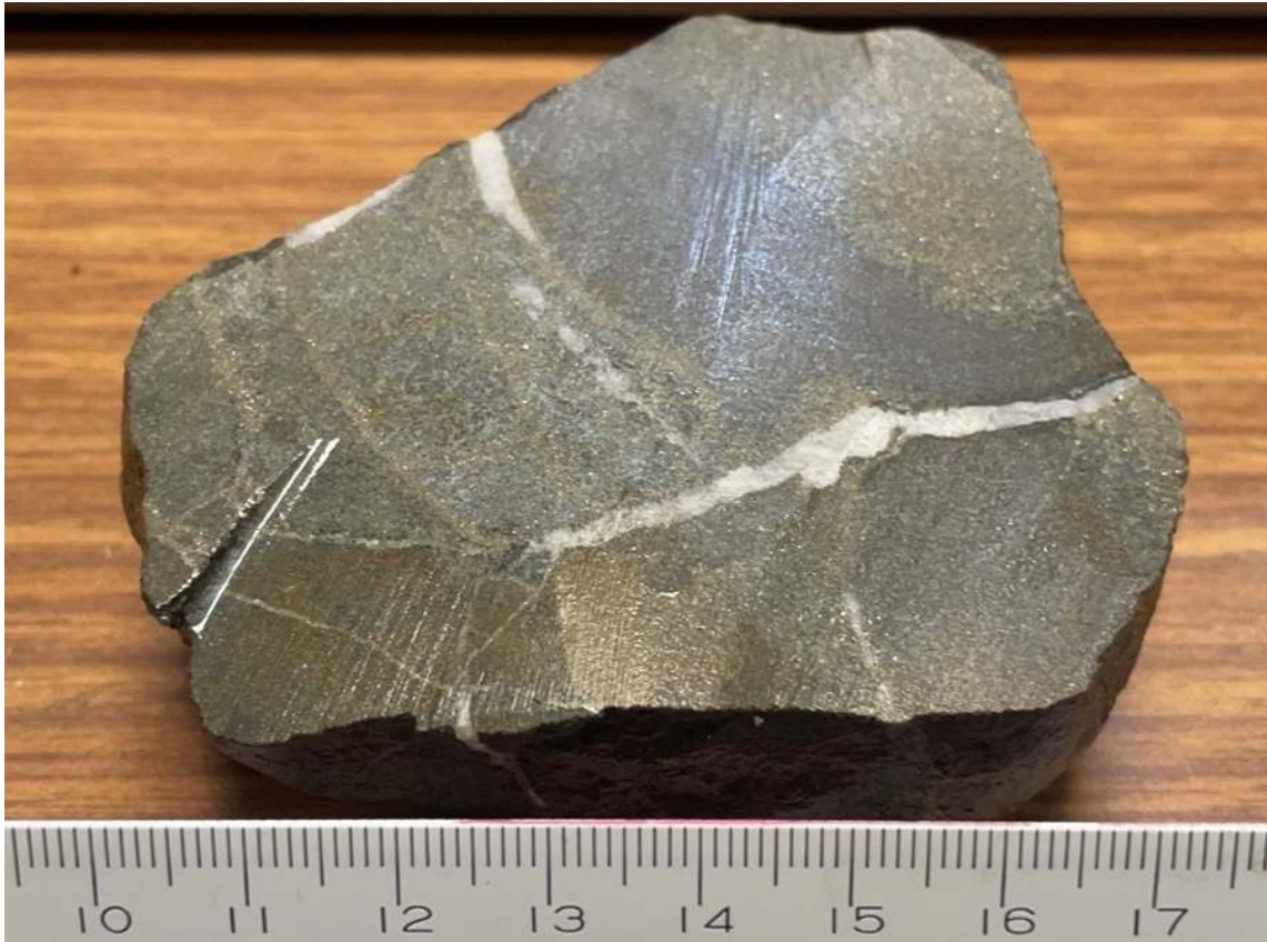
Figure 6: Cascata- Sulphide in tuffaceous siltstone.
