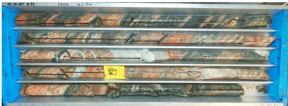
Figure 13: Potassic alteration in drill core from hole MIDD008, 162.0 - 166.25m.
