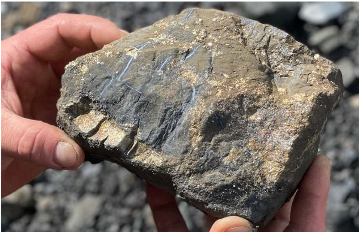
Figure 5: Cascata- Pyrite and chalcopyrite in black shale.
