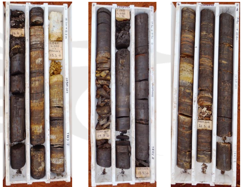
Photos: Diamond core hole OKDM002 15.1m to 19.9m. Massive manganese with minor manganiferous shale logged from 16.7m to 20.8m
