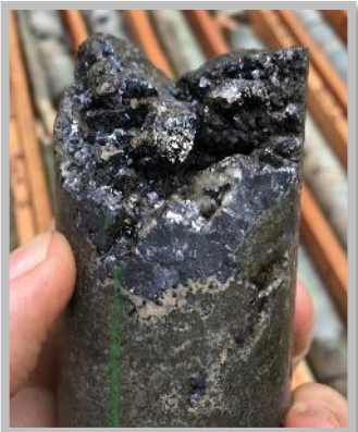
Mineralisation in hole BODD004 (2018) at Bouambo West – showing coarse galena and sphalerite within a breccia unit
