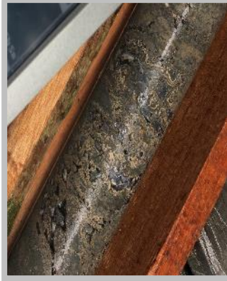
Mineralisation in hole NKDD001 (2018) at Niambokamba North – showing concentric textured sphalerite and coarse galena within a breccia unit
