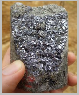
Mineralisation in hole DKDD006 (2018) at Dikaki – showing fracture-fill coarse galena within sandstone unit
