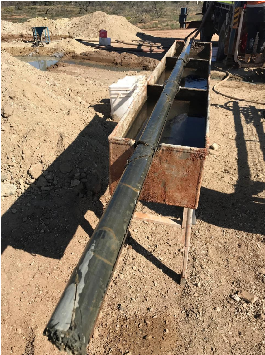
Figure 3. First Stick of Diamond Core at Worrumba 19, Showing Good Core Recovery in the Tapley Hill Formation which Overlies the Target Tindelpina Shale Unit.
