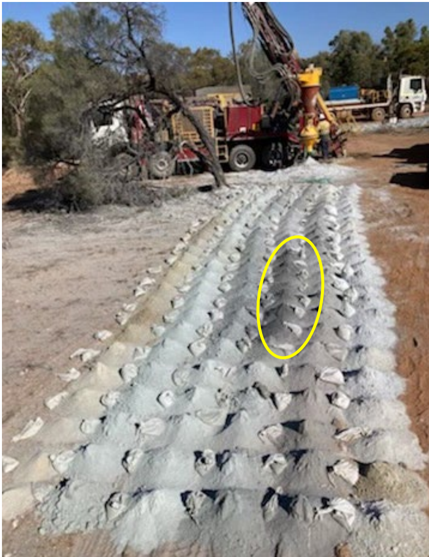
Image 2: Photo showing RC drill rig and samples from IVRC022 at the Ida Valley Gold Project, ~9m sulphide mineralisation circled.
