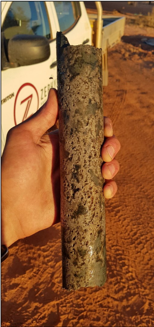
Figure 6: Section of semi-massive nickel sulphide intersected in TED14. This particular length of core is from 297.78 – 298.06m downhole. See text for further details.
