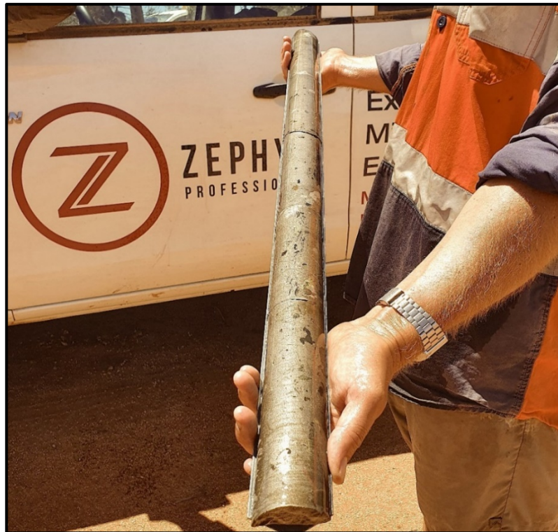
Figure 4: Photo of massive nickel sulphide in drill core of diamond hole TED07 at Dusty 1 – this part of the core grades 4.01% nickel.
