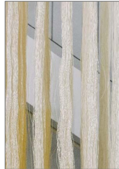
IMAGE: Hollow-fibre Nanofiltration membranes made by De.mem in Singapore
