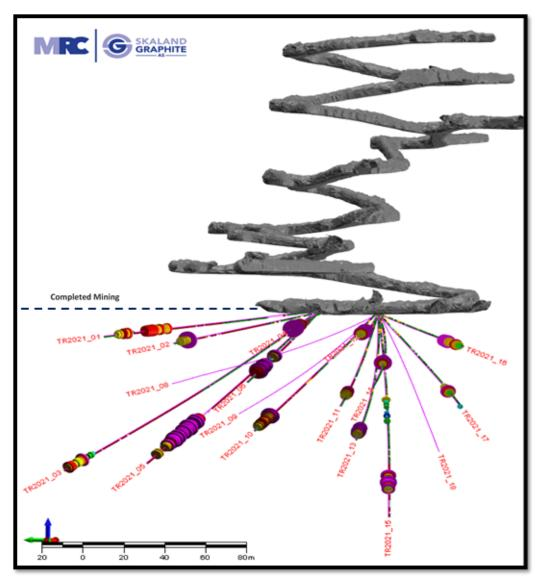
Figure 1 – Long cross section of Trælen Graphite Mine (view to east) showing graphite intersected from level +25 fanned diamond drilling in down dip
