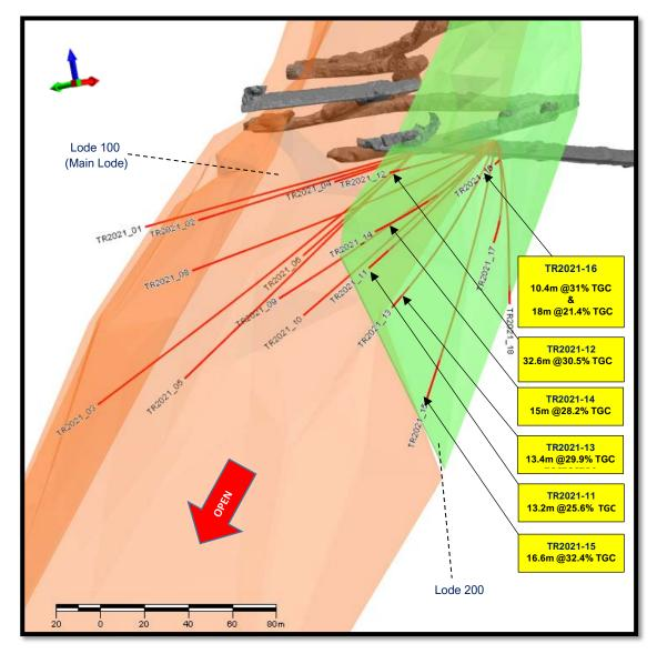
Figure 2 – View of long section of Trælen Graphite Mine showing assay results from the new 6 diamond holes
