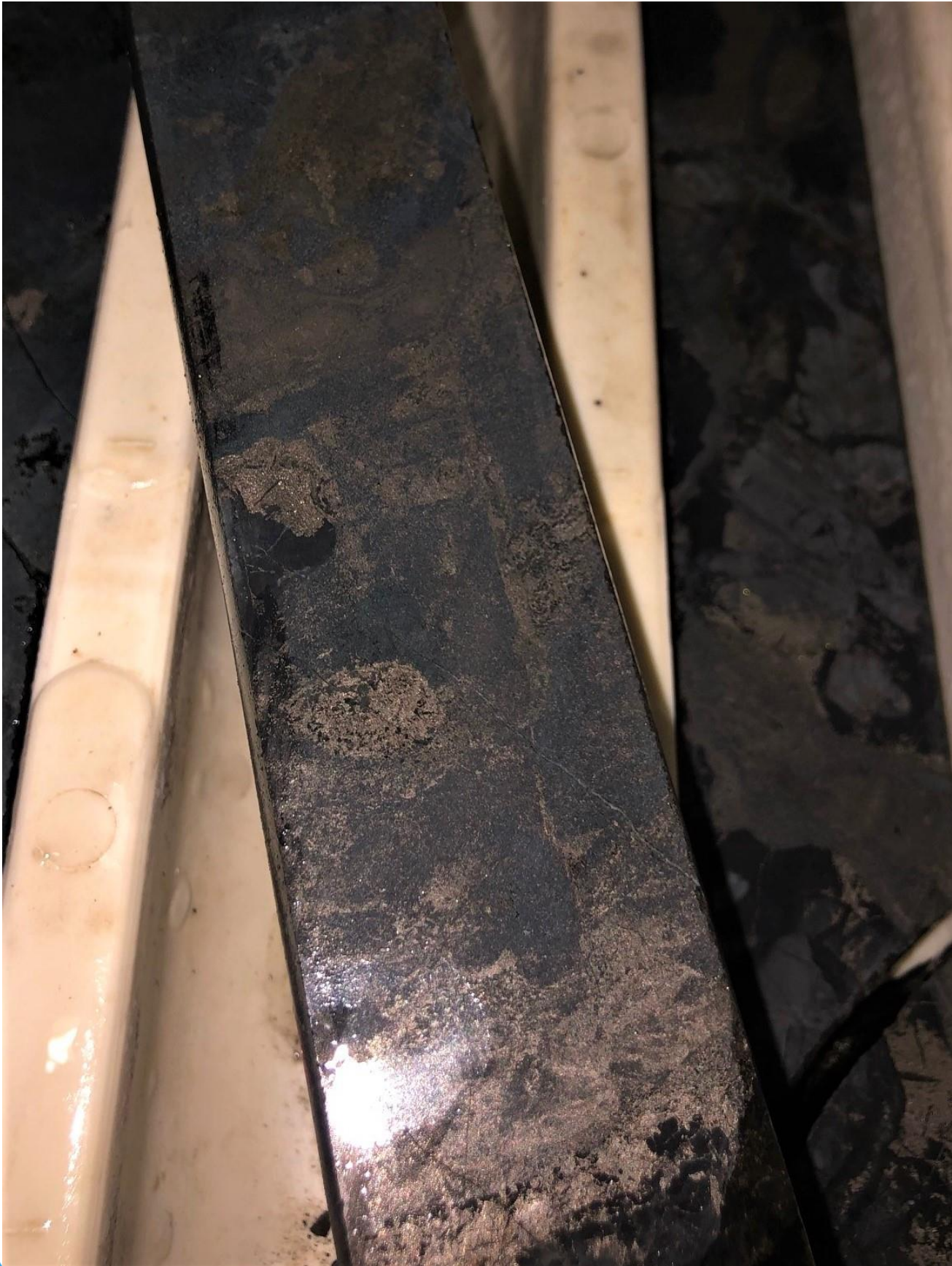
Figure One | Photo of sulfide rich magnetite skarn in drill core from 245.4m in ML337
