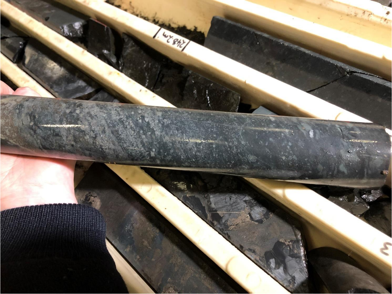
Figure Two | Photo of sulfide rich magnetite skarn in drill core from 248m in ML337
