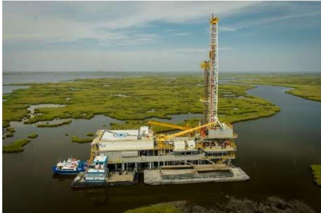
*Shallow-draft barge drilling rig*
