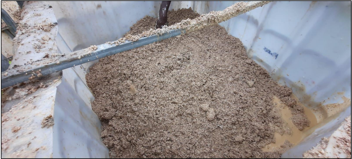
Figure 2 - Minbos Resources Cabinda run of mine high-grade phosphate rock, being extracted as part of the bulk sample.
