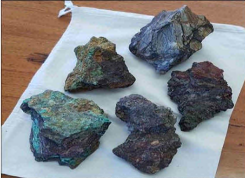
Figure 4-5: Rock samples from the Enrico Copper Mine in EL 6427, close to the Mount Dutton Fault Note: Samples show visible copper mineralisation in foliated and brecciated iron-rich rocks. Source: Copper Search
