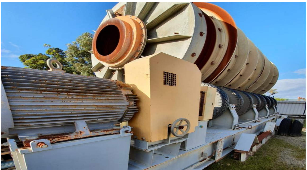
Figure 7: Wiltails Project Tailings Scrubber
