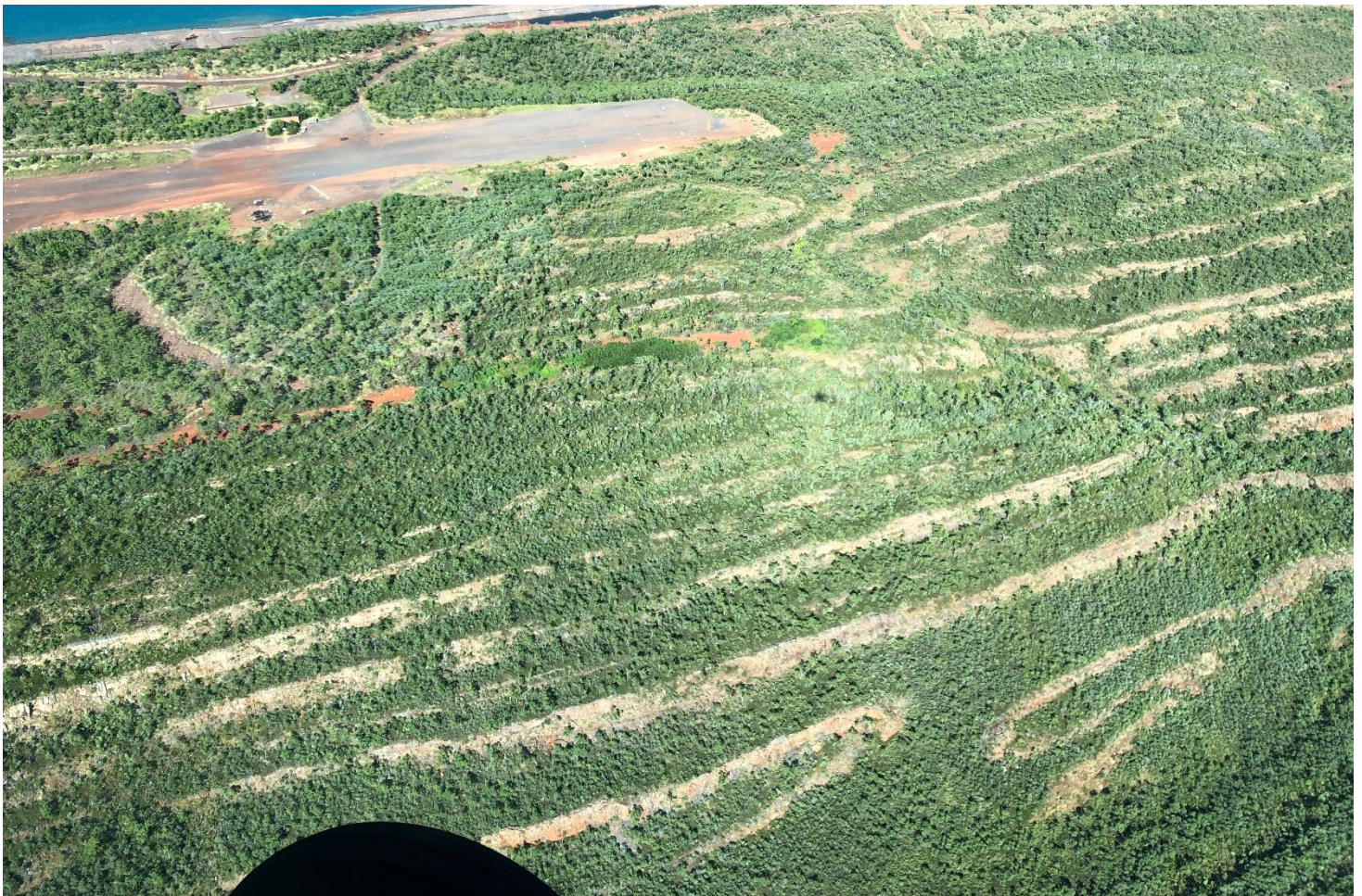
Photograph of the parasitic folding associated with the anticline on the northern portion of Cockatoo Island. It is this series of folds that delineate the approximate position of the fold axis that is the target of future exploration to the east of the North Bay target.
