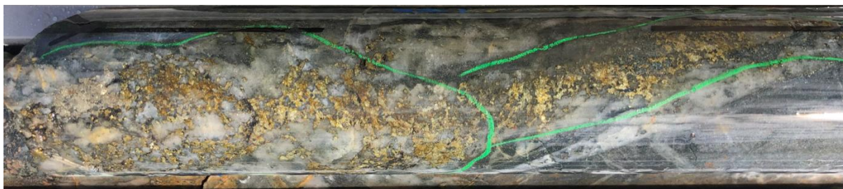
Photograph 1: Vein chalcopryrite and pyrite from 32.7m in drill hole BLDD003.
