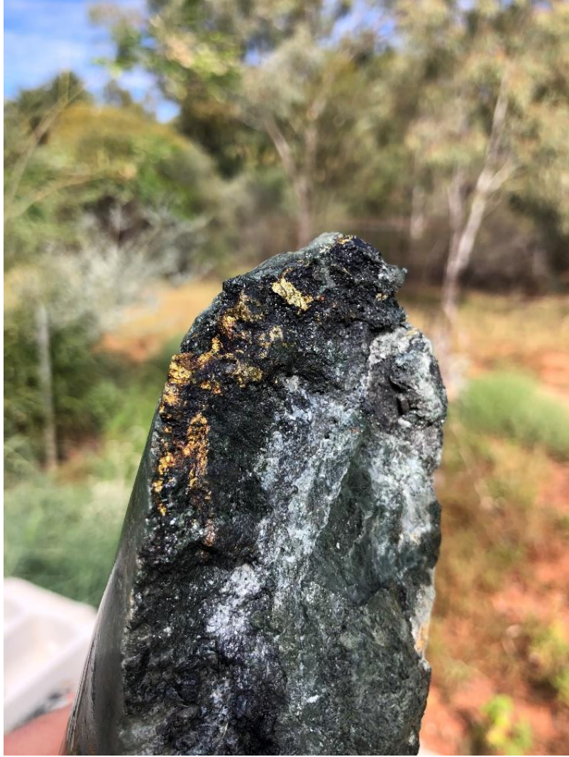
Photograph 2: Vein and fracture-fill chalcopyrite and chalcocite from 23.5m in drill hole BLDD003.
