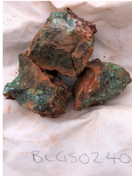
Photographs 3 and 4: Outcropping mineralisation at the newly discovered Green Hills Prospect and rock chip sample BLGS0240 which returned results of 24.30% Cu and 0.59 g/t Au.
