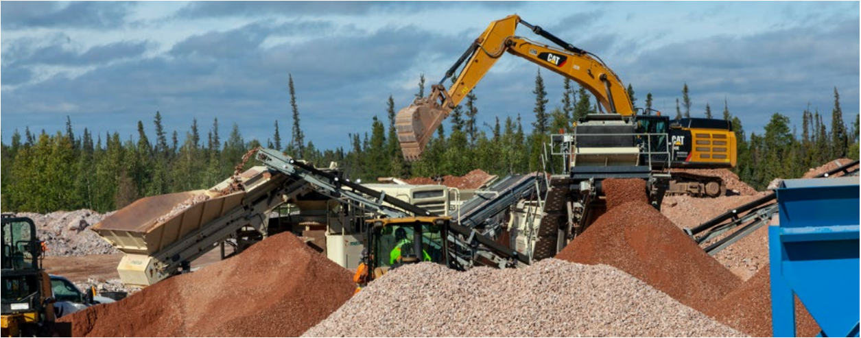
Crushing high grade ore. The red of the bastnaesite is clearly visible
