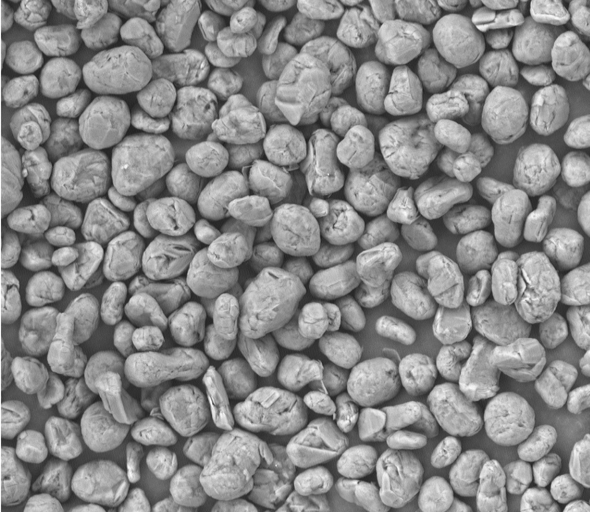
Picture 1: SEM image of 20 micron spherical graphite
