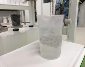
Figure 14: Core sample being weighed in air (left) and waxed core being weighed in water (right)
