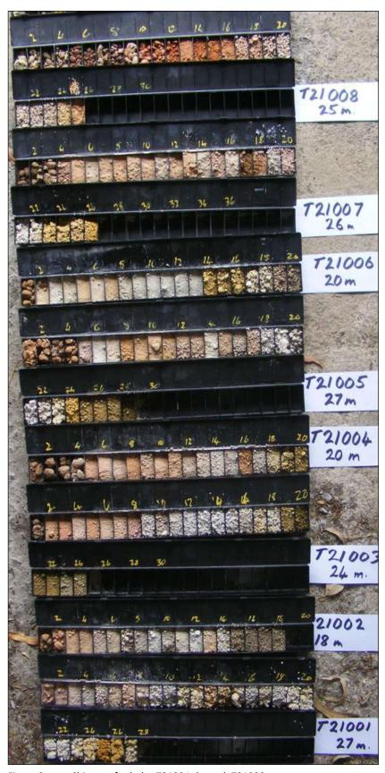
Figure 3: Chip tray for holes T21001 through T21008
