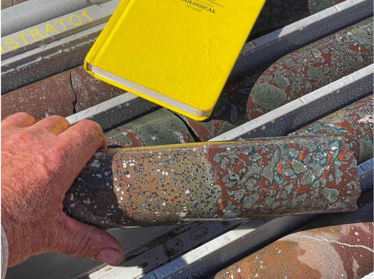
Figure 3. Diamond drill core from the stratigraphic drill hole
