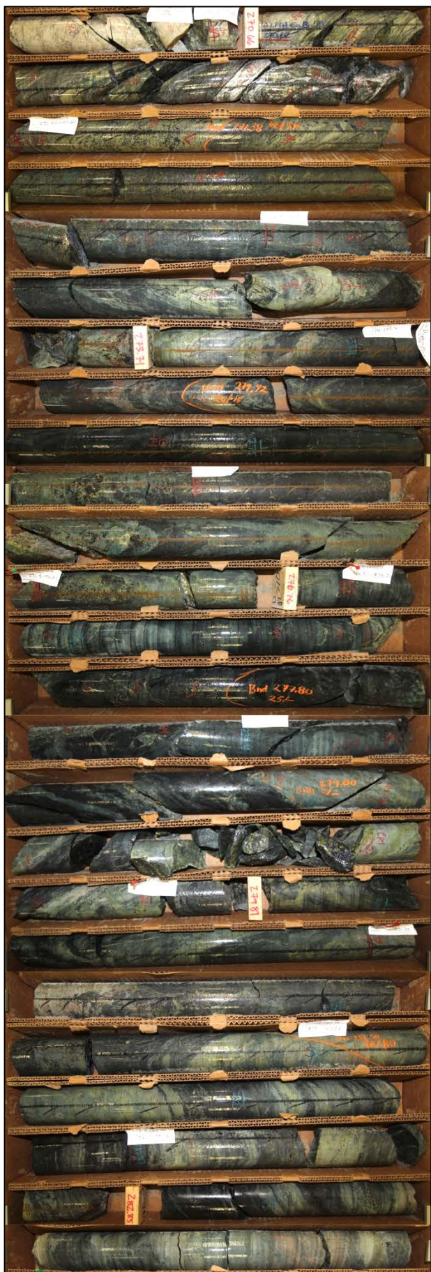
Figure 1 – Left, 13.2m strongly mineralised upper zone in drill hole WT-21-32 (270.6 to 283.8m). Right, spectacular copper mineralisation with disseminated bornite (blue) and chalcopyrite (yellow) in skarnified sediments also in drill hole WT-21-32 (272.1 to 272.5m)
