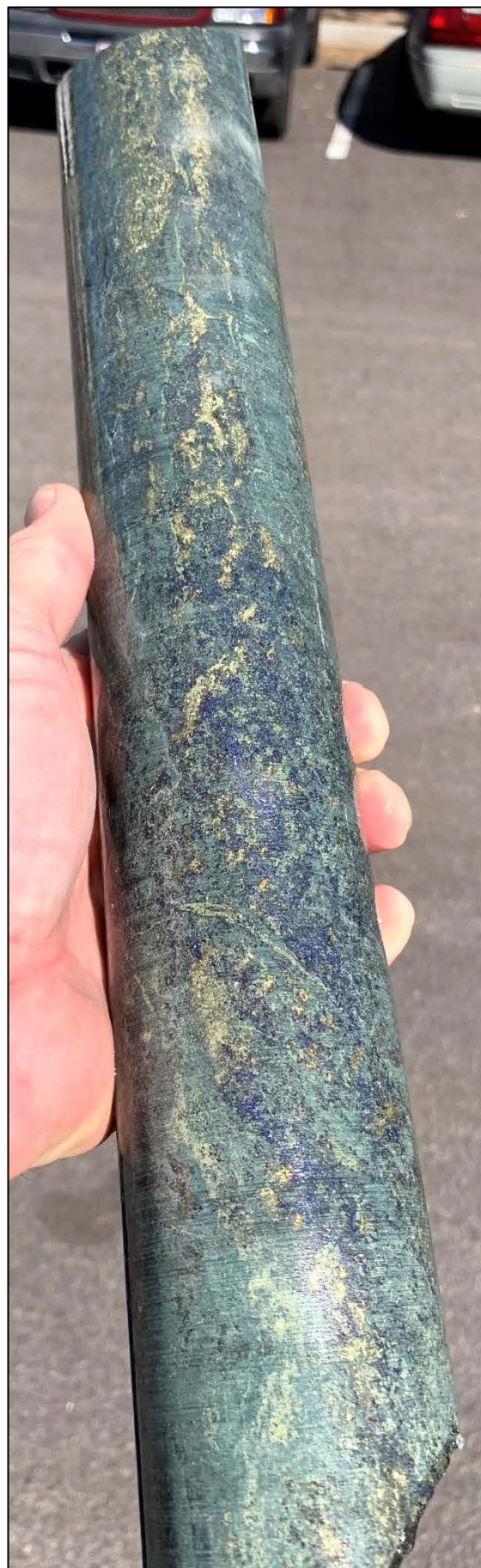
Figure 1 – Left, 13.2m strongly mineralised upper zone in drill hole WT-21-32 (270.6 to 283.8m). Right, spectacular copper mineralisation with disseminated bornite (blue) and chalcopyrite (yellow) in skarnified sediments also in drill hole WT-21-32 (272.1 to 272.5m)
