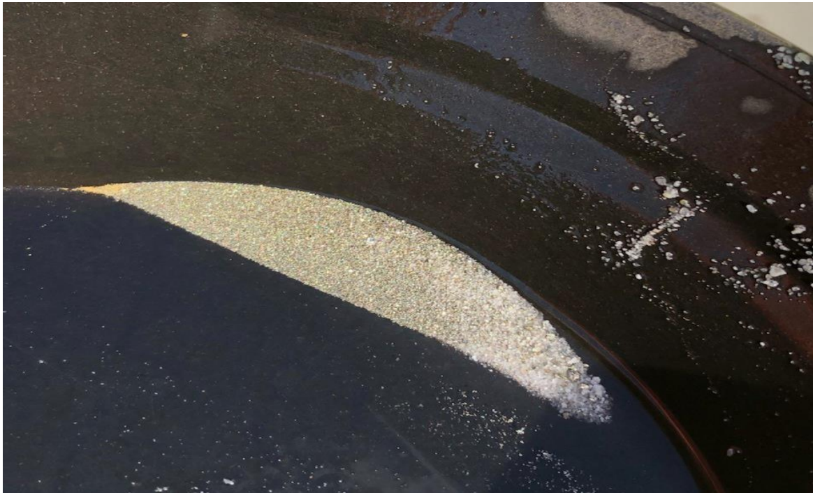
Photograph 2: PTORC022 154-155m panned visible gold
