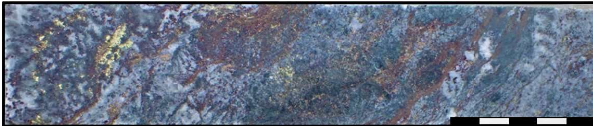
Picture 3: Drill core from KIODD004 (127m) – chlorite-actinolite-pyrrhotite-sphalerite-chalcopryite-quartz-carbonate-epidote zone.
