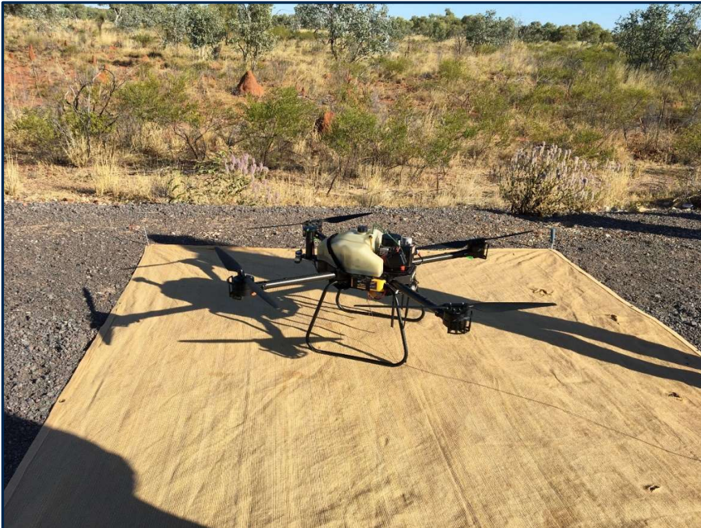
Picture 2: Recent Ultra-high resolution unmanned aerial vehicle (UAV) magnetic survey (drone survey) by Emmerson Resources in progress.
