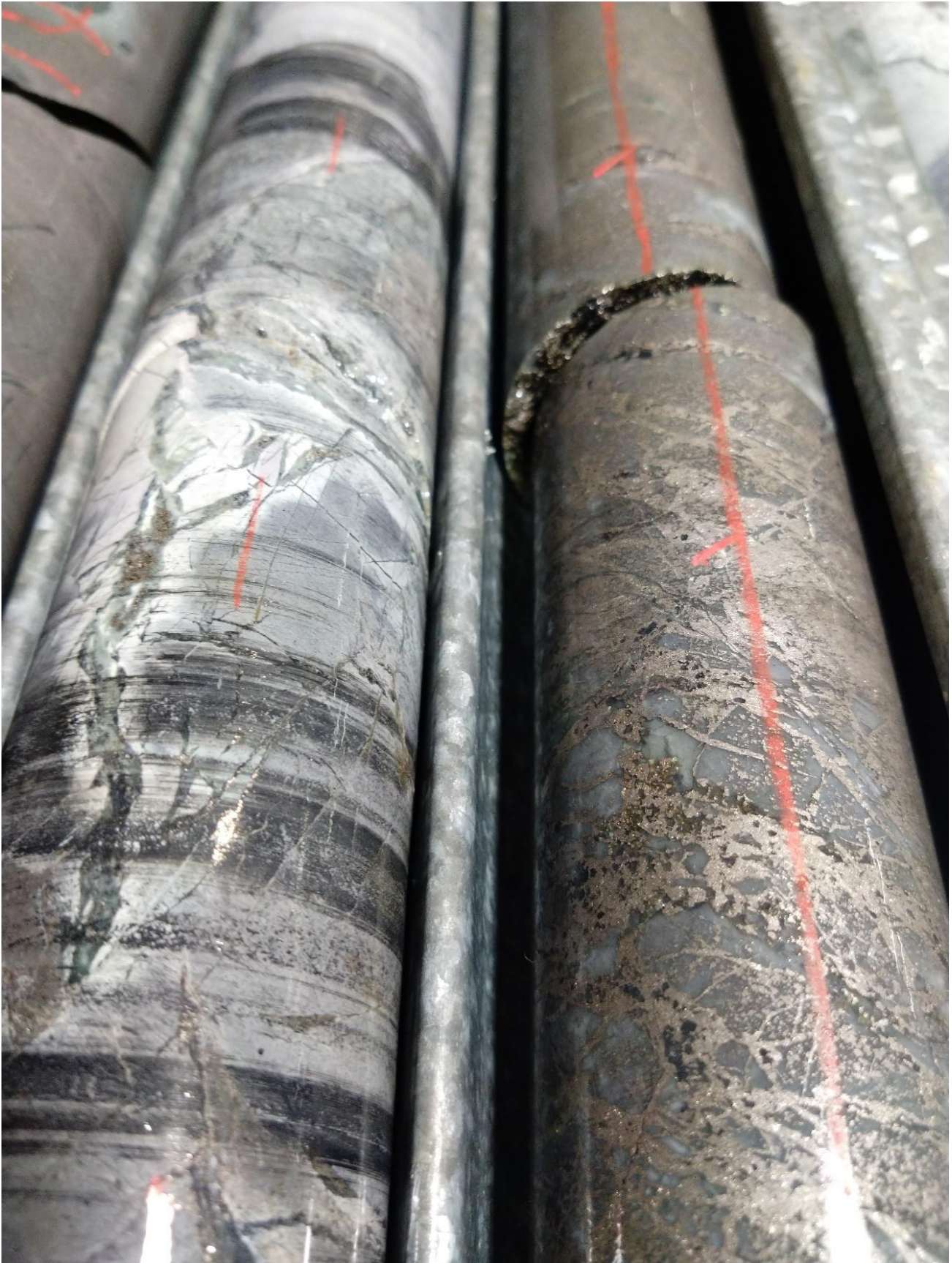
Figure One | Photo of sulfide rich skarn in drill core from 405m in ML338
