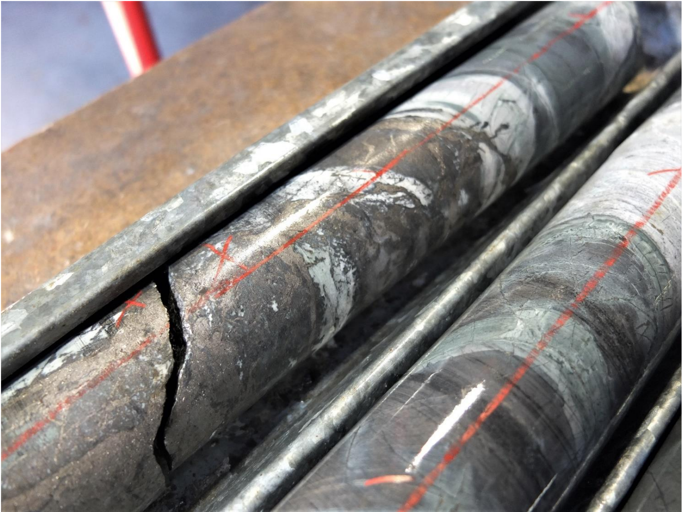
Figure Two | Photo of sulfide rich skarn in drill core from 395.8m in ML338
