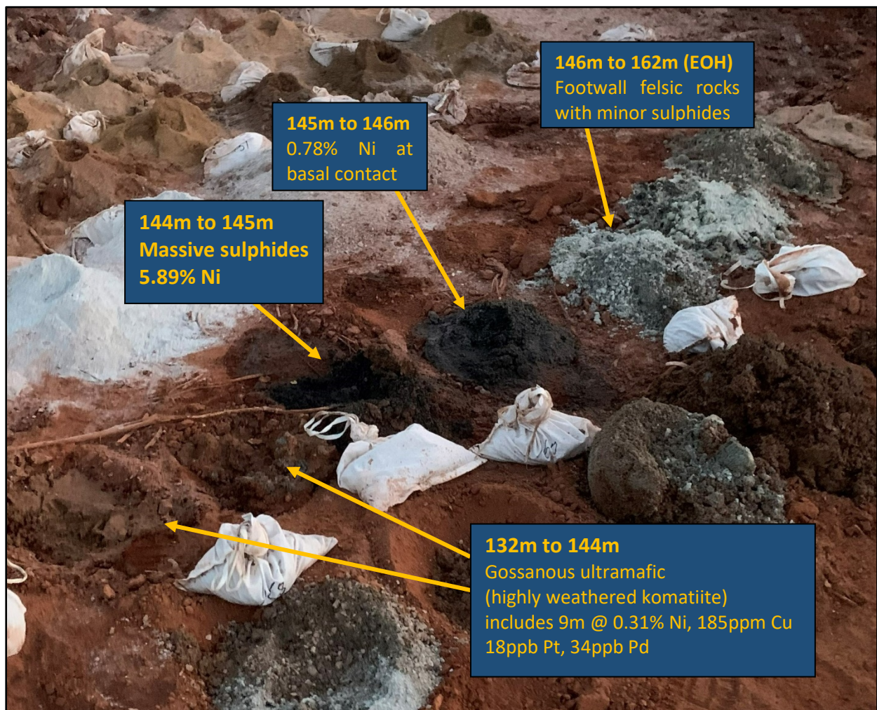
Figure 1. BVNC002 samples– nickel sulphide mineralisation highlighted
