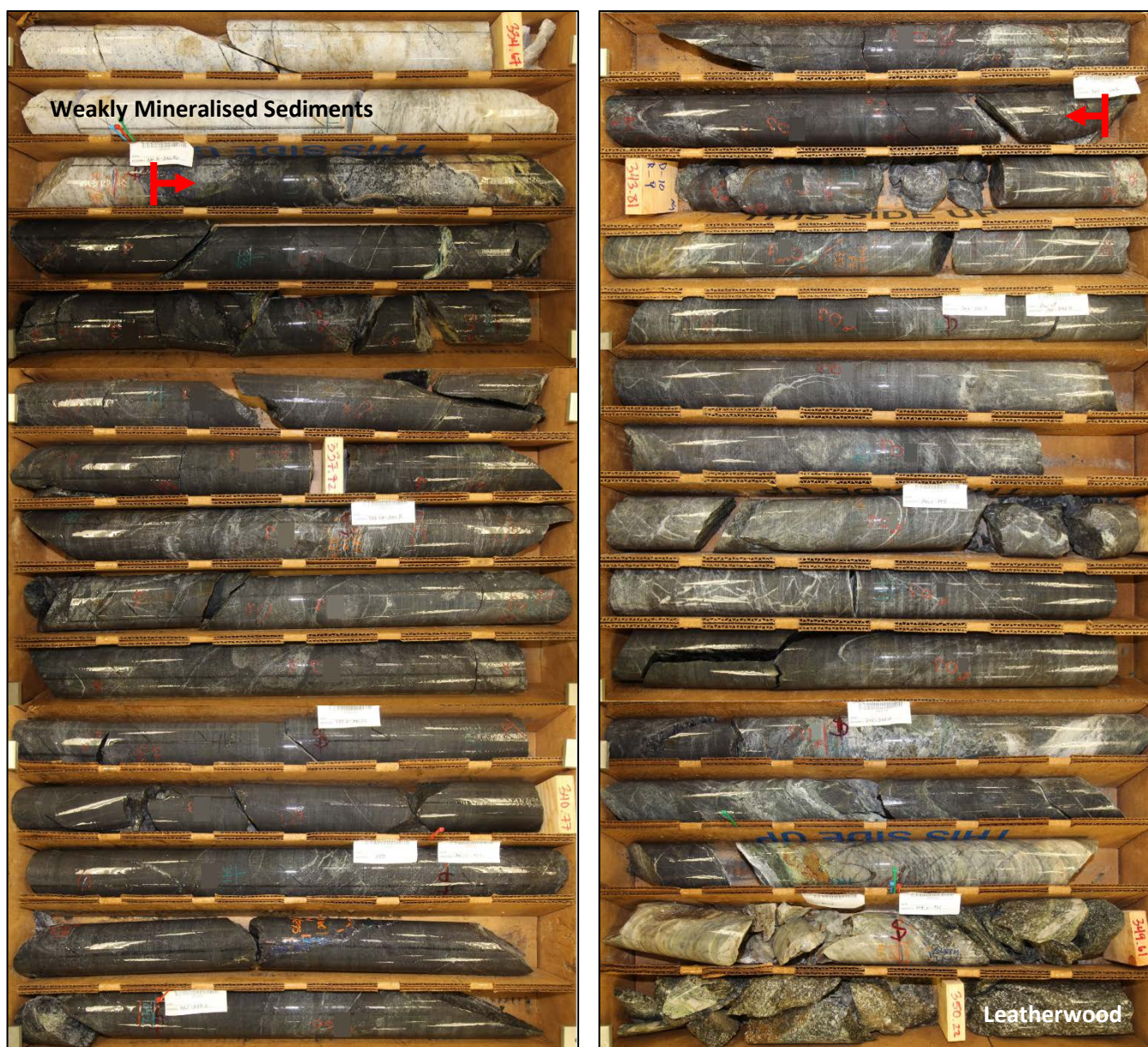
Figure 2 – 9.7m of strongly mineralised skarn in drill hole WT-21-31 (335.3 to 345m, red arrows). This interval returned 3.39% Cu, 29.65g/t Ag and 0.67g/t Au. Note colour contrast between dark grey-blue, magnetite-rich mineralisation, white unmineralized sediments (top left) and Leatherwood intrusive (bottom right). The section between 345m and the Leatherwood contact returned moderate mineralisation between 0.5 and 1% Cu. This is the lowermost of the five high-grade zones encountered in WT-21-31.
